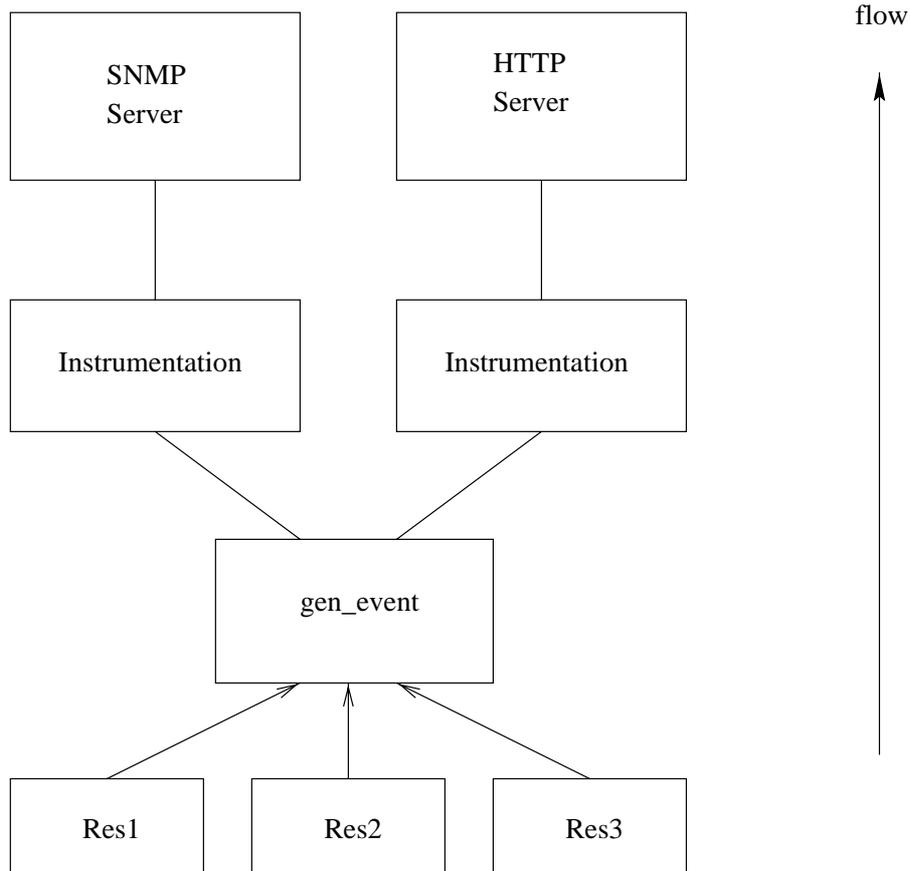
Figure 1.4: Notification handling
