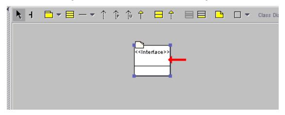
and type a name for it (like TestInterface in this case). Press "Enter# when the name is complete. (You could also enter the name by going to the Properties Tab in the Details Pane after adding the interface.)
