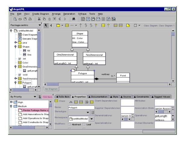
At the top of screen is a menu bar. Under that there are Toolbars. Then the bulk of the window comprises four sub-windows or Panes. Clockwise from top left these are the Explorer, Editing Pane, Details Pane and To-Do Pane. At the top of the Editing Pane is another toolbar called the Edit Pane Toolbar. Finally at the bottom of the window is a status bar.
