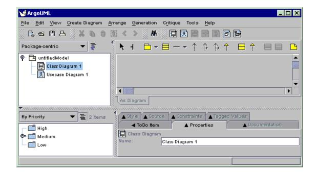
The main window's client area, below the menu and toolbar, is subdivided into four panes. Starting at the leftmost top pane, and working around the clock, you can see the Explorer, showing a tree view of your UML model, the Editing Pane with its toolbar, two scroll bars and gray drawing area, the Details Pane with the ToDoItem tab selected, and the To-Do Pane with a tree view of the to do items, ranked in various ways selected via the drop down list at the top of the pane.
