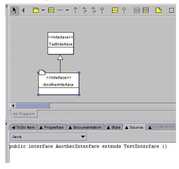
Figure 5.4. Generalization between two Interfaces.
