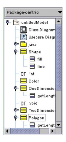
This is the explorer, where we can navigate through our model. This pane list all the classes, interfaces and data types of our model as a tree view.
