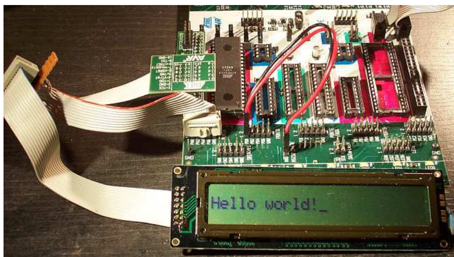
Figure 9: Wiring of the STK500
