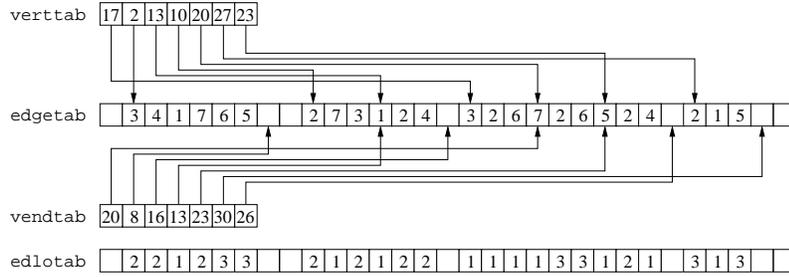
Figure 17: Adjacency structure of the sample graph of Figure 16 with disjoint edge and edge load arrays. Both `verttab` and `vendtab` are of size `vertnbr`. This allows for the handling of dynamic graphs, the structure of which can evolve with time.
