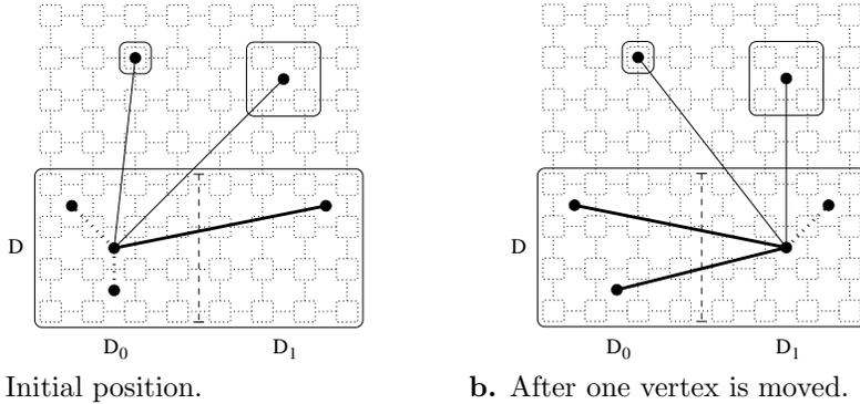
Figure 1: Edges accounted for in the partial communication cost function when bipartitioning the subgraph associated with domain  $D$  between the two subdomains  $D_0$  and  $D_1$  of  $D$ . Dotted edges are of dilation zero, their two ends being mapped onto the same subdomain. Thin edges are cocycle edges.
