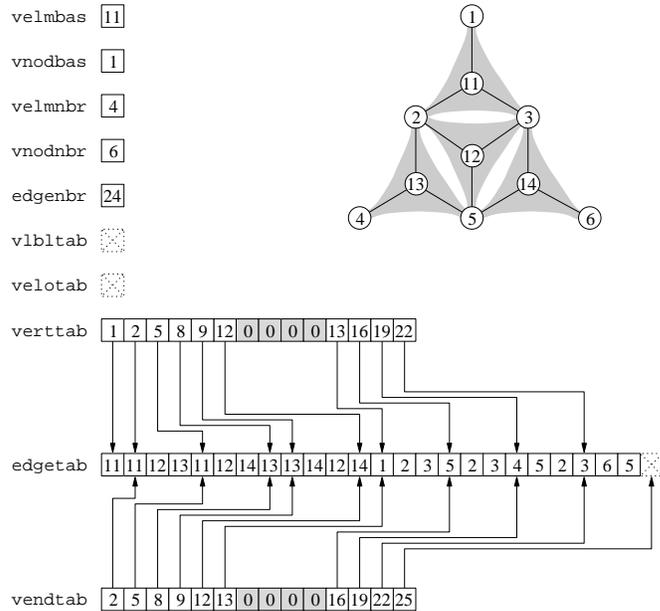
Figure 19: Sample mesh and its description by LIBSCOTCH arrays, with nodes numbered first and elements numbered last. In order to allow for dynamic remeshing, empty elements (in grey) have been inserted between existing node and element vertices.
