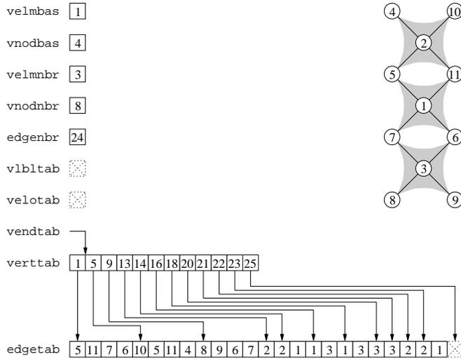
Figure 18: Sample mesh and its description by LIBSCOTCH arrays using a compact edge array. Numbers within vertices are vertex indices. Since the edge array is compact, `verttab` is of size `vertnbr + 1` and `vendtab` points to `verttab + 1`.
