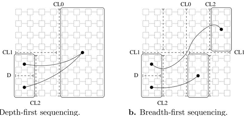
Figure 2: Influence of depth-first and breadth-first sequencings on the bipartitioning of a domain  $D$  belonging to the leftmost branch of the bipartitioning tree. With breadth-first sequencing, the partial mapping data regarding vertices belonging to the right branches of the bipartitioning tree are more accurate (C.L. stands for “Cut Level”).
