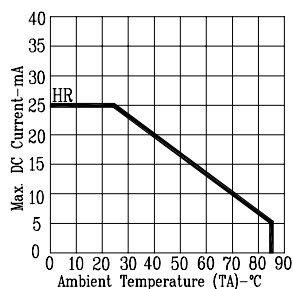
Fig5. MAX. ALLOWABLE DC CURRENT VS. AMBIENT TEMPERATURE.
