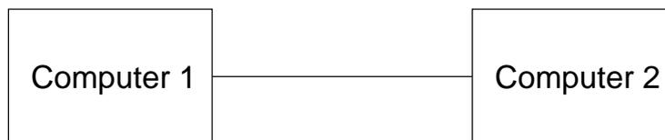
If computer 1 fails, computer 2 notices the failure and corrects the error.
