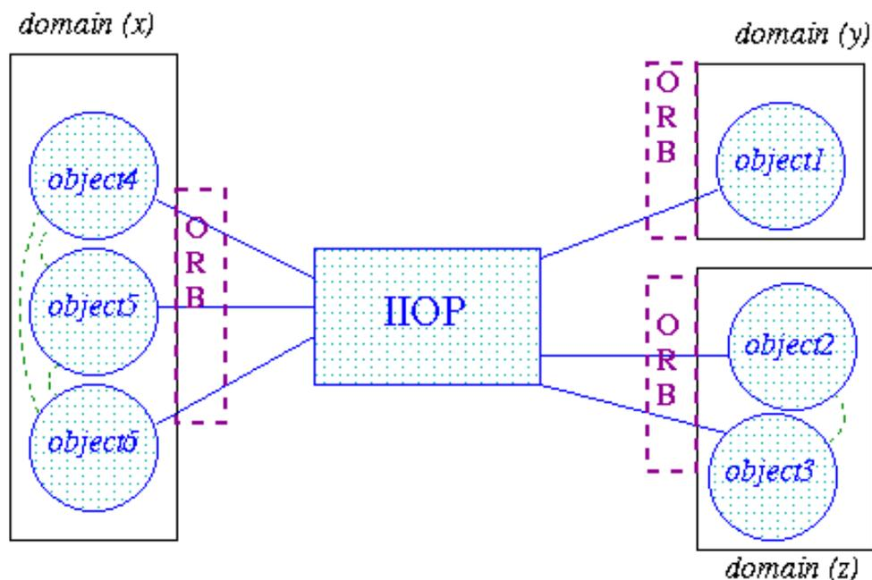
Figure 2.4: Figure 2: IIOP communication between domains and objects.
