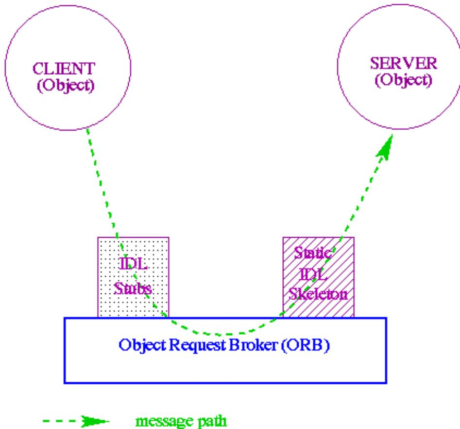
Figure 2.3: Figure 1: How the Object Request Broker works.
