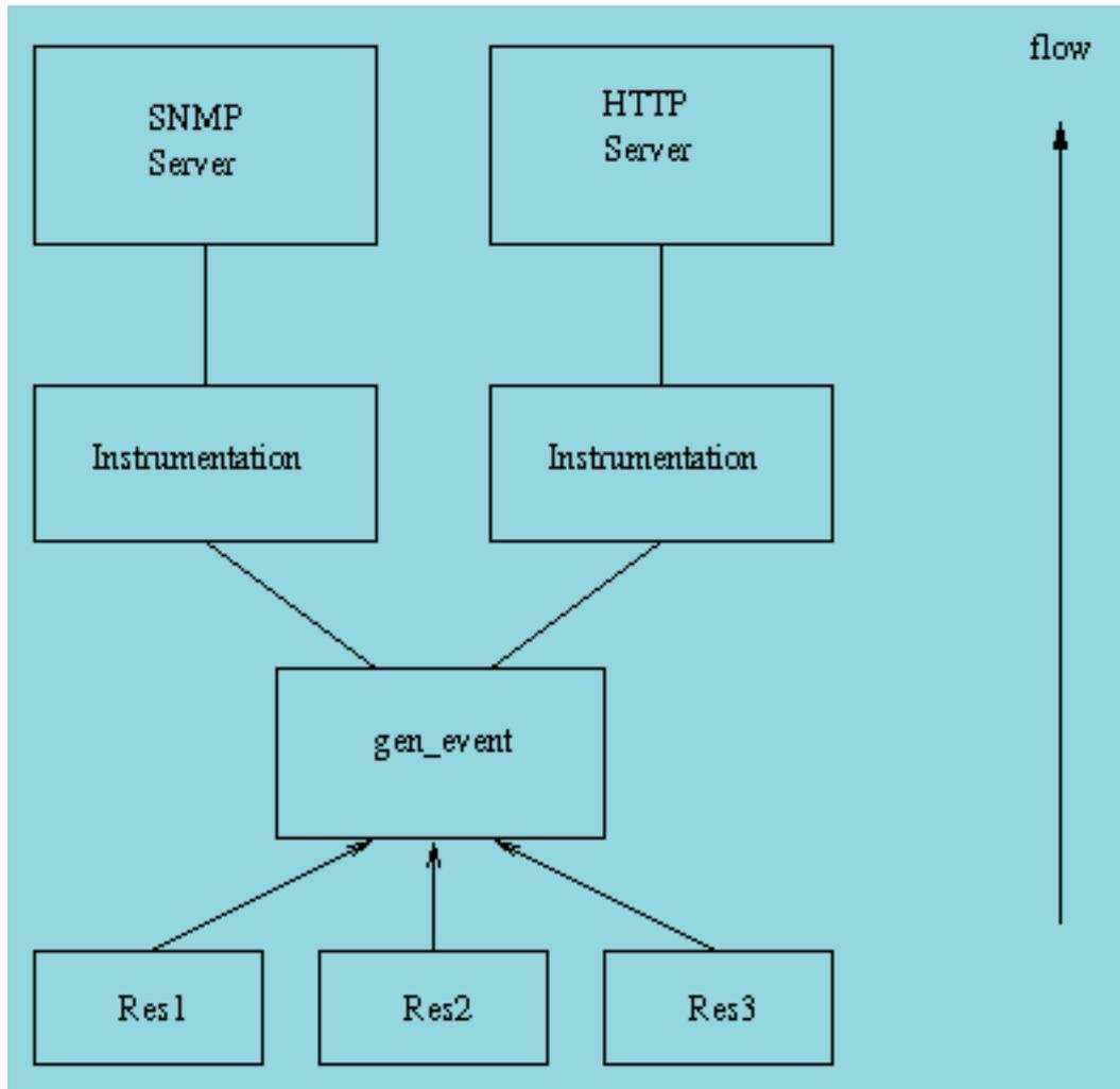
Figure 1.4: Notification handling
