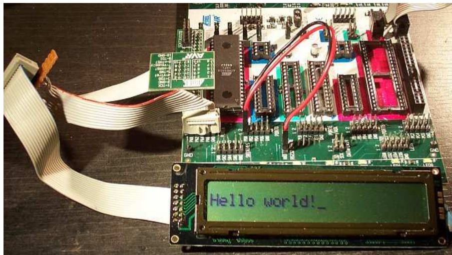
Figure 9: Wiring of the STK500
