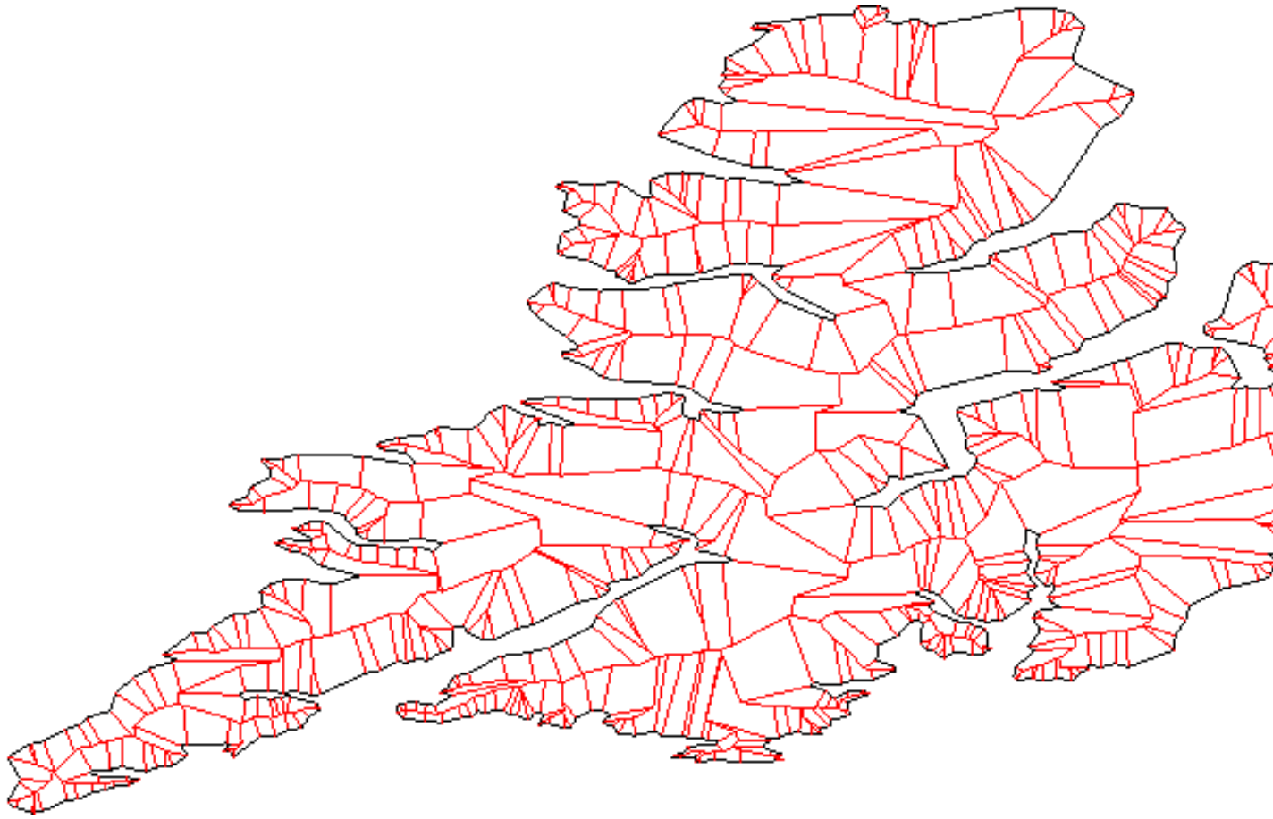
Figure 23.4: Straight skeleton of a complex shaggy contour
