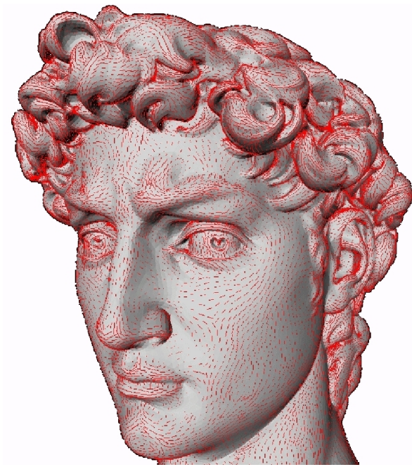
Figure 55.1: Principal directions associated with k_{max} scaled by k_{min} .
