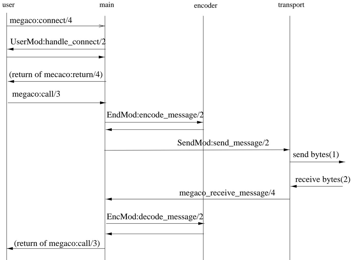
Figure 1.7: MG Startup Call Flow
