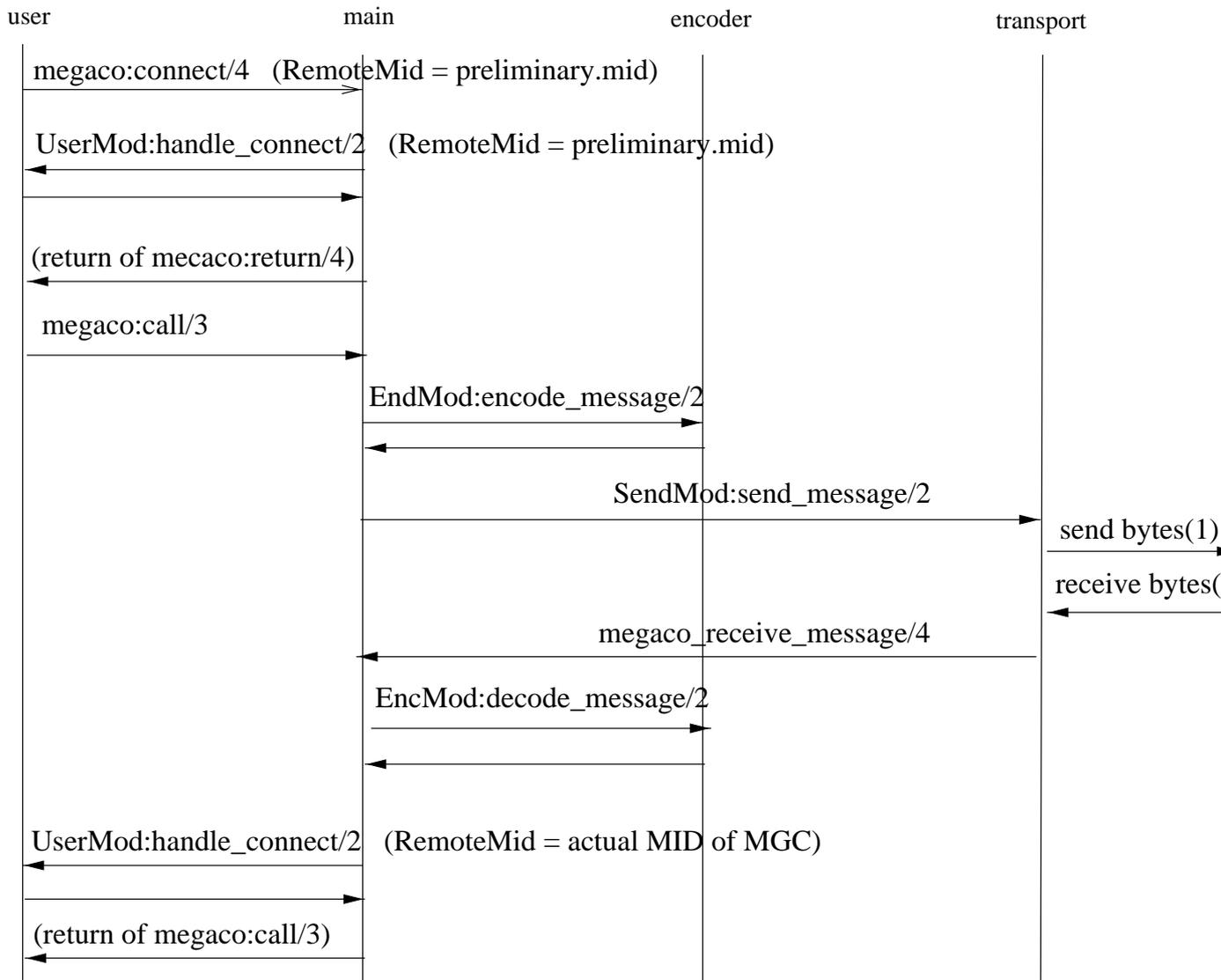
Figure 1.8: MG Startup Call Flow (no MID)
