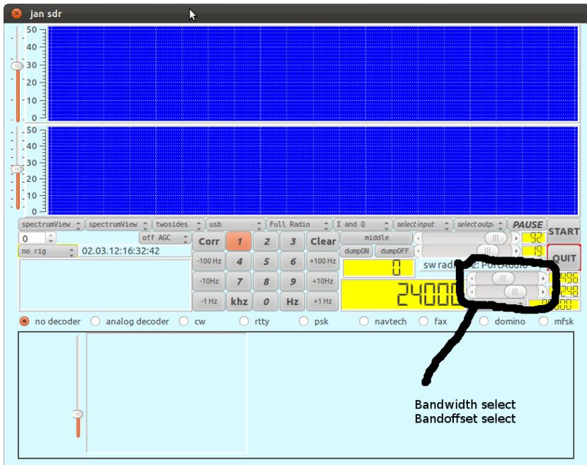
For selected devices (currently the dabstick only), there is the possibility of selecting an *offset*. Consider an upconverter that converts the frequencyband from 0 .. 30 MHz to 116 to 146 Mhz. Setting the offset to 116000 KHz allows the user to choose frequencies in the range 0 .. 30 MHz, while the actually tuned frequency is 116 MHz higher.
