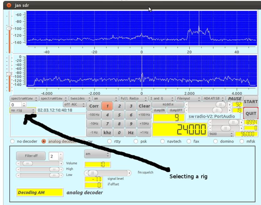
Essential is that when choosing a real device, the selected device is physically connected through the USB. On selection, the program is starting communication with the device and the device cannot be found, or cannot be opened, an error message is given and the "no rig" pseudo device will be selected again.
