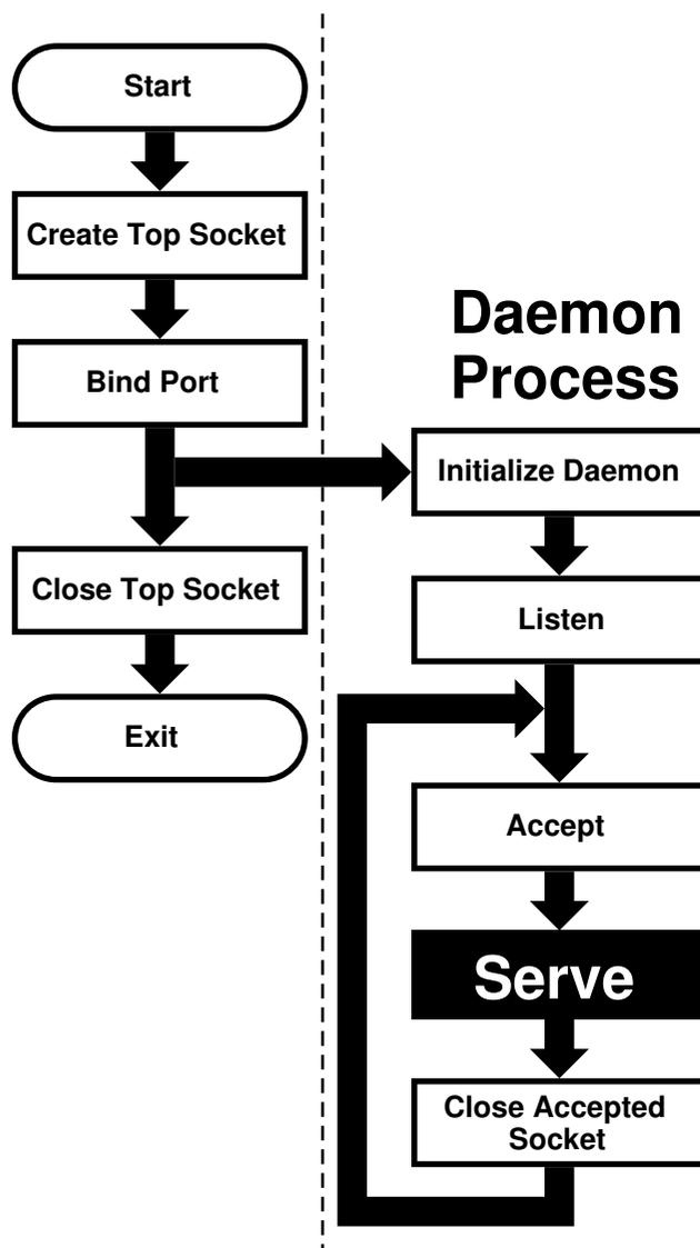
This flowchart is good for *sequential servers*, i.e., servers that can serve one client at a time, just as we were able to with our *daytime* server. This is only possible whenever there is no real “conversation” going on between the client and the server: As soon as the server detects a connection to the client, it sends out some data and closes the connection. The entire operation may take nanoseconds, and it is finished.
