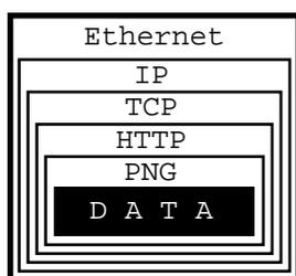
In this example, we are trying to get an image from a web page we are connected to via an Ethernet.
