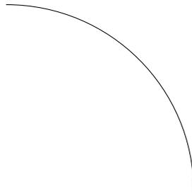
A general arc centered on `c` with radius `r` from `angle1` to `angle2` degrees (drawing counterclockwise if `angle2 >= angle1`) can be constructed with
