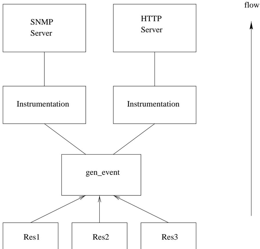
Figure 1.4: Notification handling
